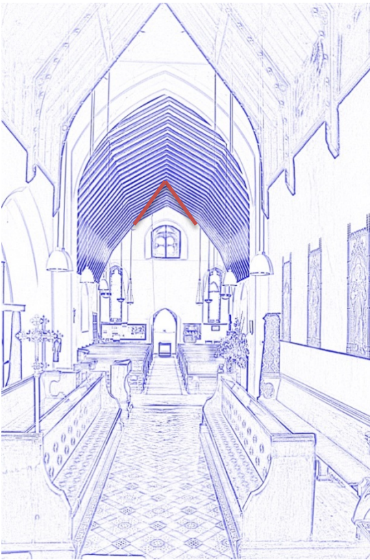
Figure 1: Cross section through the Nave showing the extended rafters above the exposed ceiling
